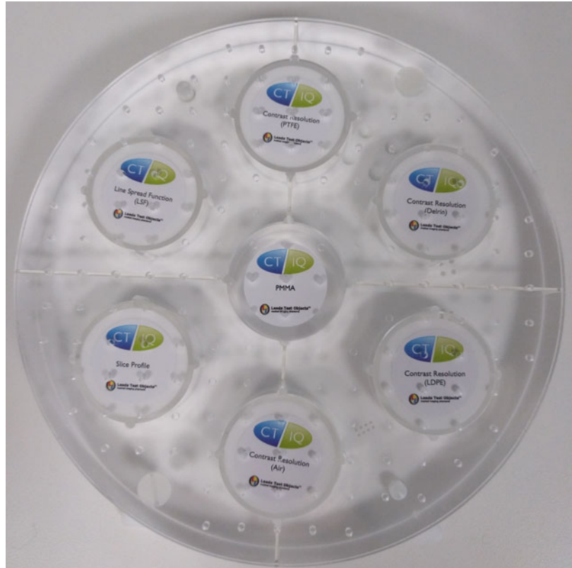
Fig. 16.3 CT imaging phantom for the study of Hounsfield unit performance (Leeds Test objects, Leeds, UK)
